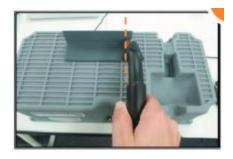
2. Place the end of the MIG on the right edge of the T-Joint at a 45° angle. Press the trigger and release.
